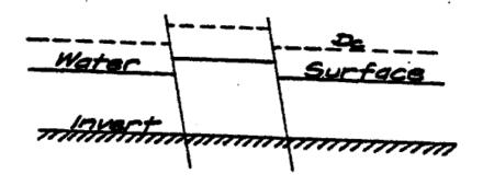
(d) If, at the upstream end of the pier, no depth can be found to balance the P + M equation, calculate P + M for the depth of flow just outside the upstream end of the pier and its sequent depth. If the lower stage results in the greater sum (P + M), this indicates a hydraulic jump at the upstream face of the pier. If the upper stage results in the greater sum (P + M), this indicates a hydraulic jump at the upstream face of the pier.
