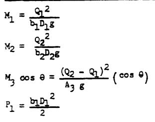
Where  $A_3 =$  water area at section 3  $P_2 = \frac{b_2 D_2^2}{2}$   $P_1 = \left(\frac{b_1 + b_2}{2}\right) = \left[D_1 + \frac{(D_2 - D_1)(b_1 + 2b_2)}{3(b_1 + b_2)}\right]$   $P_w = \frac{D_1 + D_2}{4}(b_2 - b_1)\left[D_1 + \frac{(D_2 - D_1)(D_1 + 2D_2)}{3(D_1 + D_2)}\right]$  $P_f = \frac{L(s_1 + s_2)}{4} \cdot (b_1 D_1 + b_2 D_2)$
