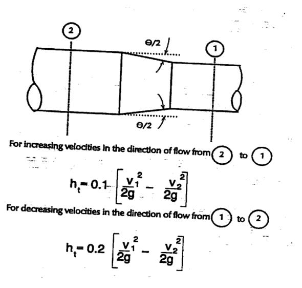
Deviations from the above criteria must be approved by the City Engineer/SSCAFCA. When such situations occur, the angle of divergence or convergence ( $\theta/2$ ) may be greater than 5 degrees 45 minutes. However, when it is increased beyond 5 degrees 45 minutes, the above equation will give results for h<sub>t</sub> that are too small, and the use of more accurate methods, such as the Gibson method shown Plate 22.3 B-2, will be acceptable.
