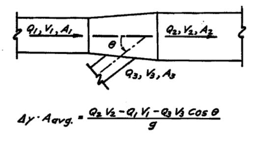
Where  $\Delta y = difference in hydraulic gradient for the two end sections, in feet$ Aavg = average area, in feet<sup>2</sup> = 1/6 (A<sub>1</sub> + 4A<sub>m</sub> + A<sub>2</sub>) or, for practical use 1/2 (A<sub>1</sub> + A<sub>2</sub>)A<sub>m</sub> = mean area of flow, in feet<sup>2</sup>
