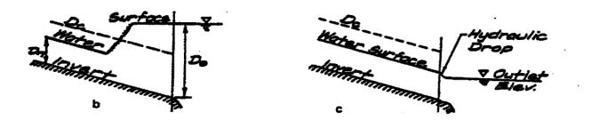
(c) Where the water surface of the outlet is below the water surface in the channel or conduit, control is upstream and the outflow will have the form of a hydraulic drop.
