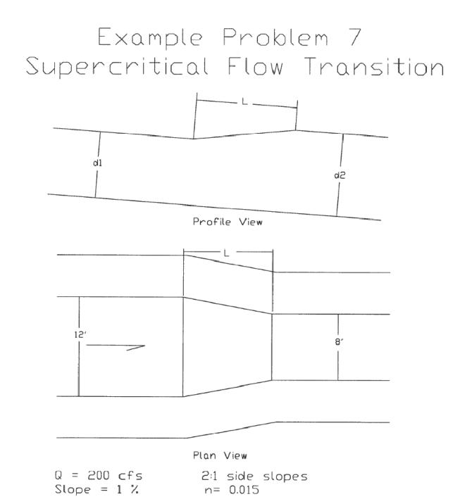
Determine the minimum length L to ensure that a hydraulic jump does not occur through the transition and that the transition angle is small enough so that oblique waves are negligible.
