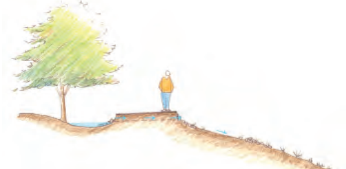
Swale along trail with shallow basin and overflow disbursement in section
