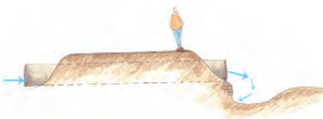
Culvert with Zuni bowl/dissipation pond device
