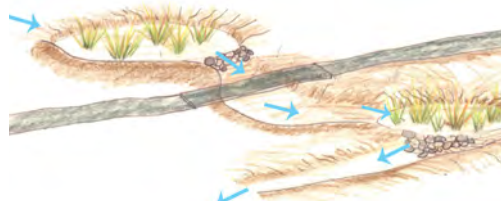
Slowing and ponding small drainages to protect trail
