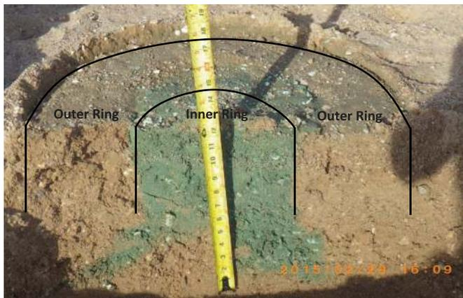
**Fig. 5.** (Color) Dye added to the inner ring of a double-ring infiltrometer showing the extent and direction of flow after removal of steel rings (tape measure scale: in inches; 1 in. = 2.54 cm) (image by author)
