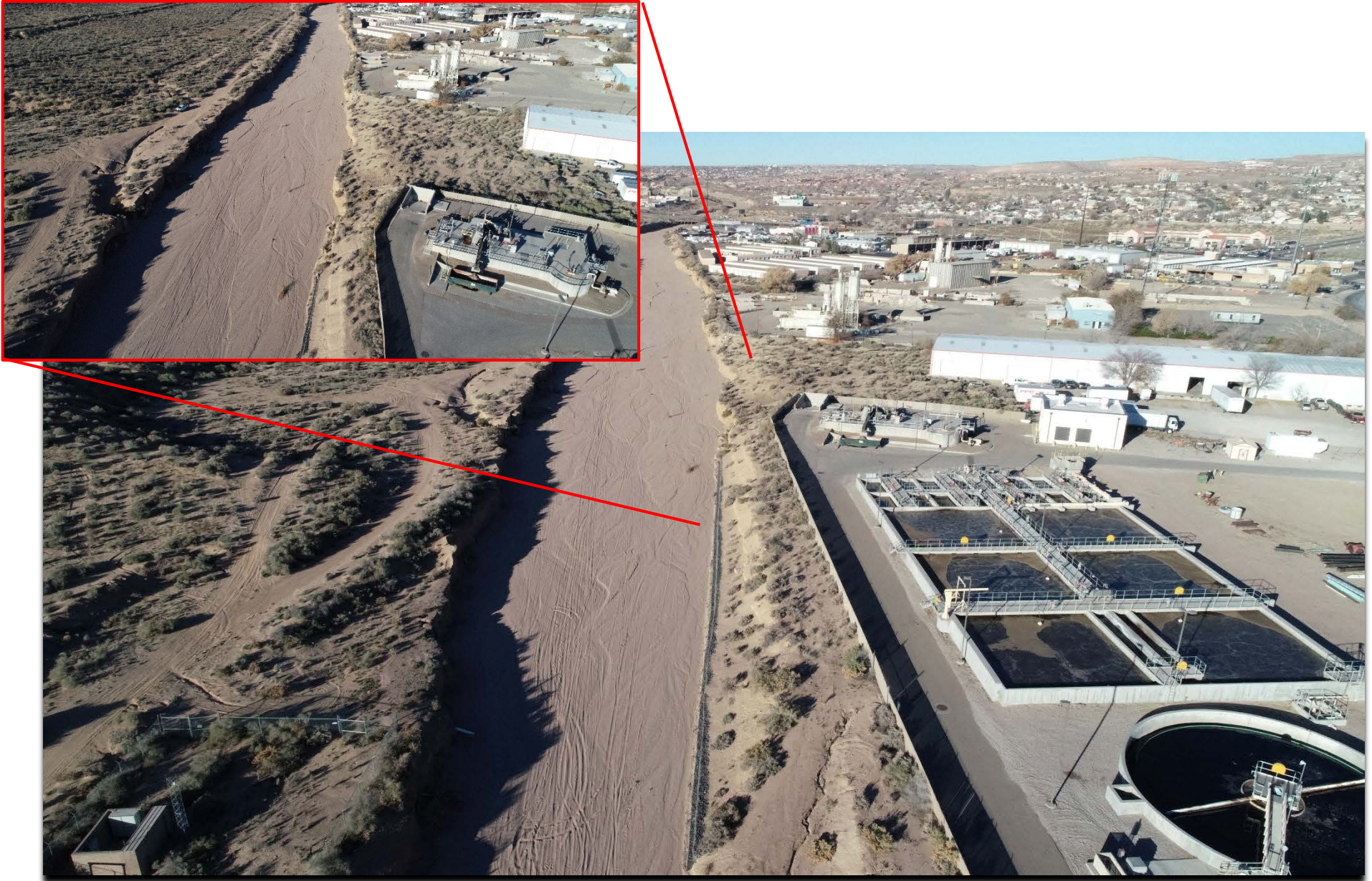
Figure 6 - Photos showing erosion cut towards headworks of WWTP.
